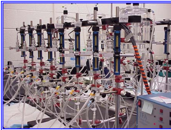
Figure 1A: Close-up view of 8-bath isolated vessel ring set up.
