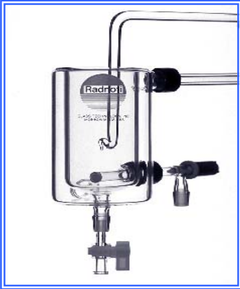
Figure 2: Close-up view of chamber for mounting aortic ring.
