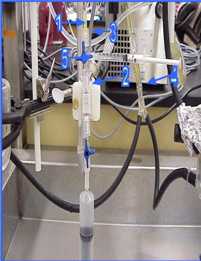
Figure 2: Close up photo of setup for preparation of balloon. Stub adaptor [1]; 3-way stop cock [2]; 1 ml syringe [3]; transducer [4]; Biomedix balloon and holder [5];
