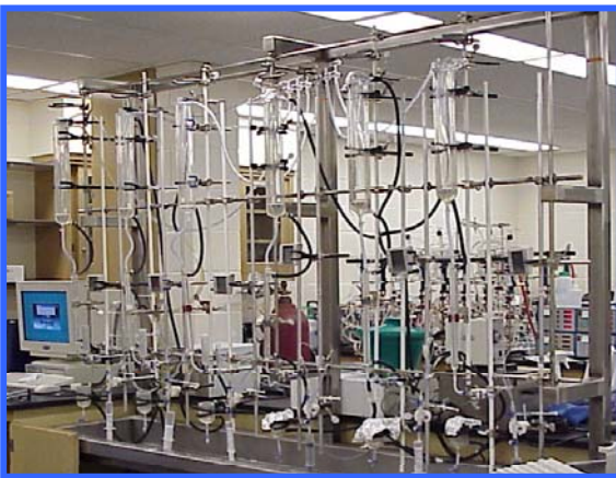
Figure 1A: View of 6 Langendorff perfusion set-ups used for high-throughput studies.
